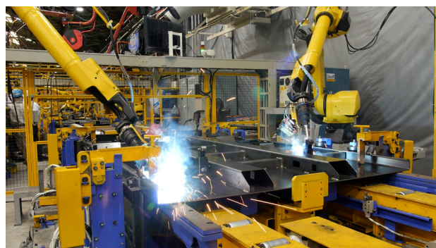
Small-sized rear dump trucks body automation line at the Yokohama plant
