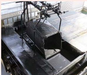
The body and tailgate are coated with an electro-deposition process to enhance rust prevention effects.
