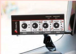
The shape of switches inside the cab have been changed and LEDs are used for the switch lamps for better control and visibility.
