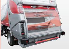
An integrated one-touch handle and inner slide cover with optimized sliding mechanism are included as standard accessories. These makes opening and closing the cover smoother, and reduces the effort required.
