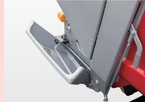
Fold-out storage pockets are built into the tailgate side covers. The fold-out design prevents objects from falling out while driving.
