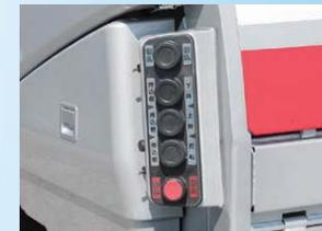
The loading switch control panel on the side of the loading hopper is angled to the rear left. This enables operation from side of the vehicle, and keeps the operator safe even with unpredictable movement of waste within the hopper.
