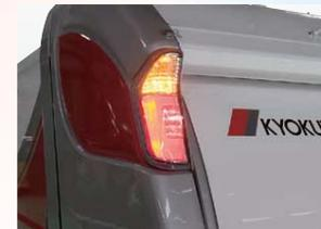
Specially designed LED rear combination lamps have been used as the tail lamps. These improve visibility both from behind and the side, making waste collection work even safer.
