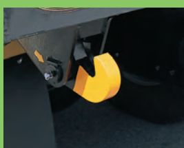
▲ Automatic tail gate locking device
