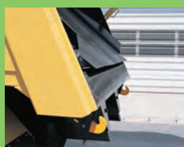
▲ Discharge plate with over stroke mechanism
