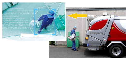
Safety support system equipped with image recognition AI for garbage trucks (This image is an image of detection. )
