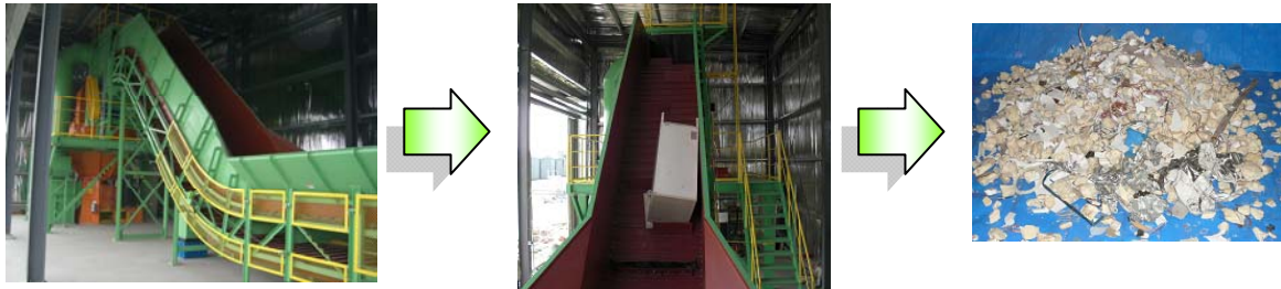
Pulverizer system for demonstration in Kunshan Plant (China)
