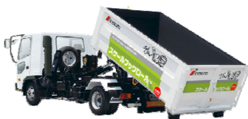
Detachable body truck equipped with scale “Scale Hook Roll”
