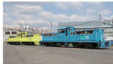
New lithium-ion battery locomotive
