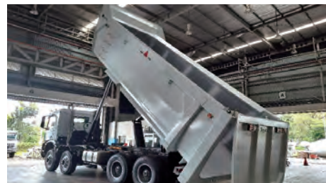
45m 3 large-capacity rear dump truck
