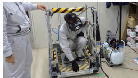
Experiencing a forklift forward/reverse accident using the VR danger experience device
