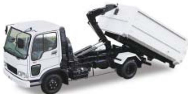
“Hook Roll” is a system of the truck with detachable bodies (containers) separable from the carrier. You can use multiple containers and realize shorter loading time, reduction of man-power, and loading cost.
