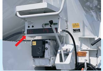
后部供水操作盘 Rear end water supply control panel
