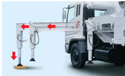
易于设置, 稳定性好的2节伸缩式前方支架 Easy setting and safe double telescopic front outriggers
