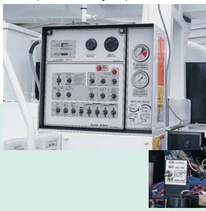
内装有高低压转换开关的控制盘 Control panel with built-in high/low pressure selector switch
