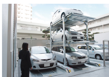
Multi-story parking equipment
