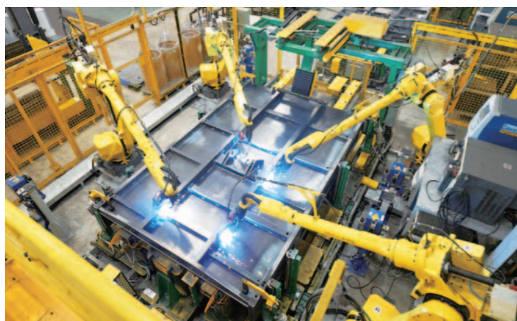
Automatic welding robot for dump truck body
