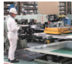
Tailgate lifter load test
